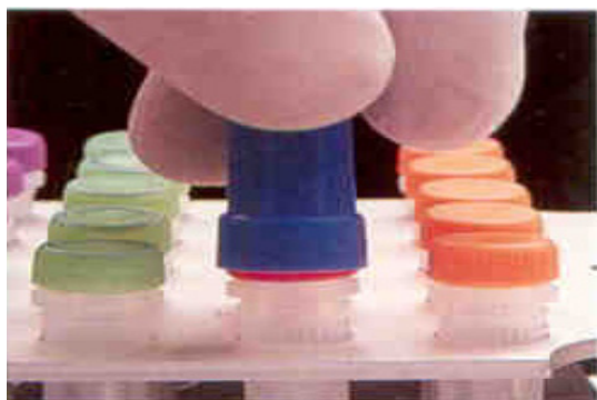
The Micro tube tool's larger end is a socket wrench for Screw-Cap Micro Tubes.
