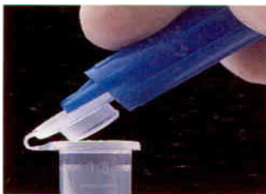
Shown: The Micro Tube tool's smaller end is used to open a Snap Cap Micro Tube.
