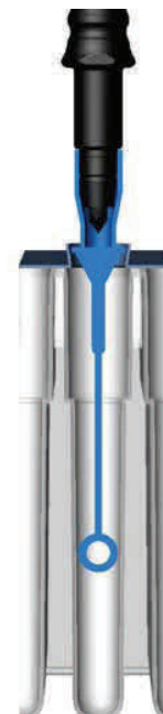
This illustration shows the three easy and rapid steps used to extract a sterilized 10uL Astral Loop from its sealed chamber.
